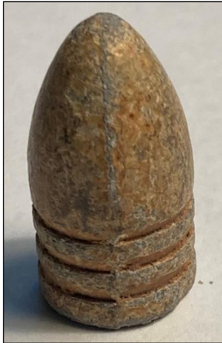
Figure 5. A .58 caliber, unfired, nose cast bullet. One of two mold seams is visible running down the length of the bullet in the middle. The sprue nib is the little gray spot on the nose of the bullet to the right of the seam. This bullet has a length of 1.02 inches, a mean diameter of 0.565 inches and a grain weight of 487.8. The cone depth is 0.335 inches. Author's collection
