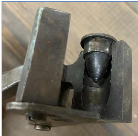
Figure 2. The same mold as shown in Figure 1, in the upside down, open position. To the right is one of two blocks containing a cavity which is half of the negative impression of a bullet to be cast. Nesting in the top of the cavity is the plug. The plug creates the cavity in the base of a bullet. The plug is removable and held in place by a plug screw. Figures 1 & 2 from SHOOTERS FORUM @. https://www.shootersforum.com/threads/how-can-i-figure-out-what-caliber-this-bullet-mold-is.240126/ .
